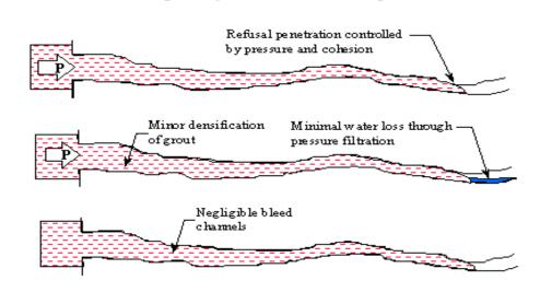
Grouting theory - balanced, stable grouts
